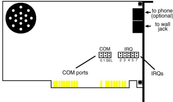
When doing a “Plug and Play” installation, the jumper shunts should be placed so that they are hanging from single jumper pins rather than on pairs of pins. Your modem’s jumper shunts should already be in this Plug and Play configuration. If they are not,
