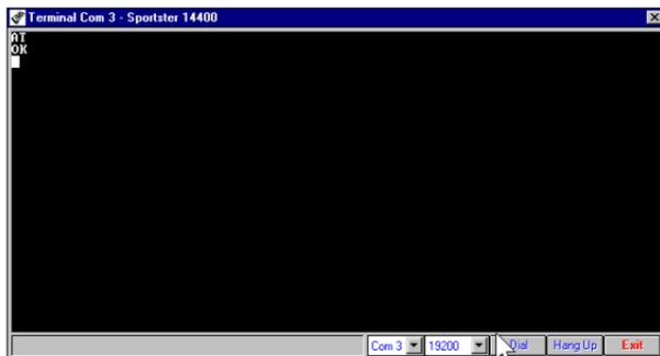
In addition to allowing direct entry of modem commands, the *Terminal* window also allows you to dial into Bulletin Boards, listing services, and other online services.
