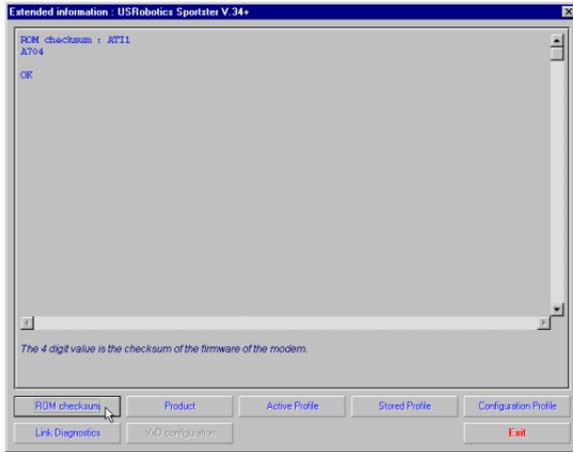
Technicians use the ROM Checksum to verify information stored in the modem's Read Only Memory. You can check the ROM Checksum from any Terminal program by typing **ATI1** and pressing **ENTER**. For information about the specific modem you are using, click **Product** to bring up the next screen.
