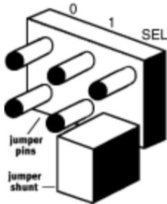
3. To change the COM port and IRQ settings, you need to reposition the jumper shunts on the COM port and IRQ pins. To do this, lift the jumper shunts off the pins.
