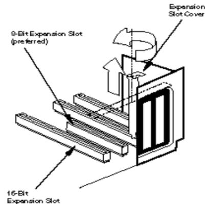
5. Holding the modem at each corner, with the gold edge facing the slot, push the modem down as gently as possible until it snaps into the expansion slot. (Note: The following diagram shows horizontally aligned expansion slots. Some computers have vertically aligned slots. The instructions apply to both styles.)
