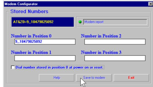
To store a number in your modem’s memory, simply click in one of the entry boxes. Type in the phone number exactly as you would dial it. NOTE: Position Zero has a special feature. You can set your modem to automatically dial this number when your computer is turned on or when it is reset.
