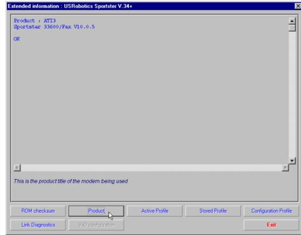
The “Product” screen displays the make and model of your modem. It is the equivalent of the ATI3 command.
