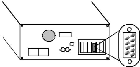
you need a shielded serial modem cable with a 9-pin female to 25-pin male connector.
