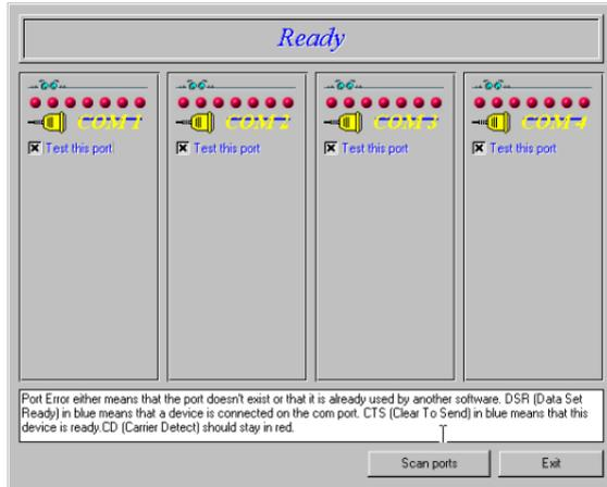
The screen consists of four columns, one for each possible COM port on a PC. You can scan a specific port(s) by selecting the checkbox for that port.
