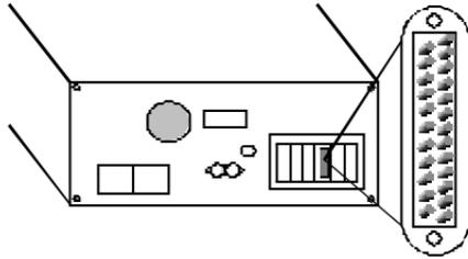
you need a shielded serial modem cable with a 25-pin female to 25-pin male connector.
