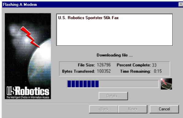
10. When the download is complete, the modem disconnects from the server. The words “Downloading file...” change to “Upgrading ...” or “Updating ...”, depending on whether you are upgrading or updating your modem. A new progress bar appears. This indicates that your modem’s code is being updated.
