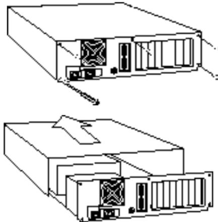
4. Find an empty ISA expansion slot that's at least as long as the gold edge of your modem. (ISA slots are black plastic grooves lined with silver.) Unscrew and remove the expansion slot cover (the long narrow piece of metal that keeps dust from entering through the opening perpendicular to the slot). Be careful not to drop the screw into the computer. You will need it later to screw the modem into place.
