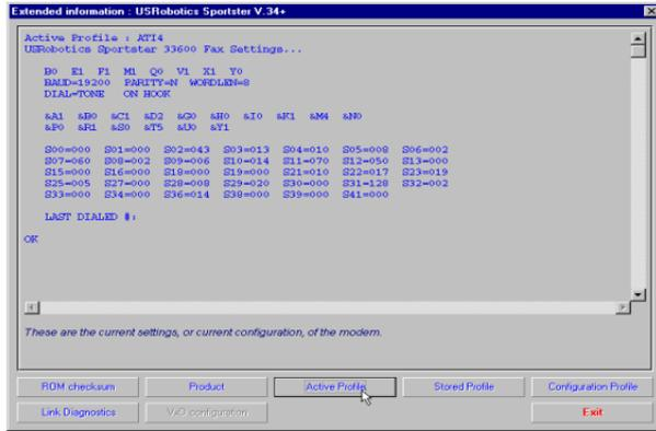
This screen contains information about your modem's current configuration. Starting from the top, you will see the make and model of your modem. Directly below that you will see basic commands currently in use. Below that are the current connection settings.
