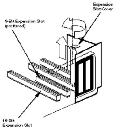
5. Holding the modem at each corner, with the gold edge facing the slot, push the modem down as gently as possible until it snaps into the expansion slot. (NOTE: The drawings show horizontally aligned expansion slots. Some computers have vertically aligned slots. The instructions apply to both styles.) You need to apply a little pressure to seat the modem properly. Sometimes a gentle back-and-forth motion helps to fit the
