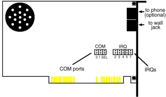
The jumper shunts will be hanging from single jumper pins as shown in the following illustration.
