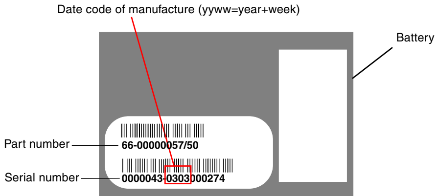
FIGURE 4-2 Battery Label Example for the Sun StorEdge 3510 FC Array
