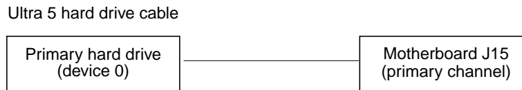
FIGURE A-2 Hard Drive Cabling Configuration (One Drive)
