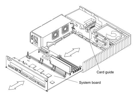
FIGURE 9-20 Removing the System Board
