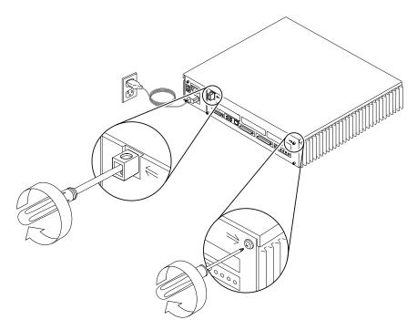
FIGURE 7-5 Securing the System Unit Cover
