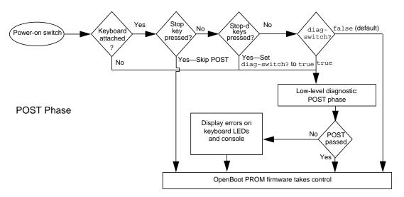
FIGURE 2-1 Factory-Defined Boot Sequence—POST Phase Settings and Tests
