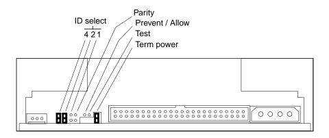
FIGURE 9-5 Jumper Settings for the CD-ROM Drive
