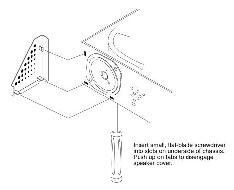
FIGURE 8-5 Removing the Speaker Cover
