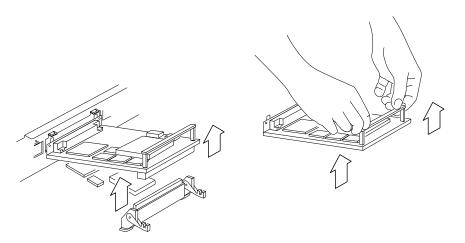
FIGURE 11-5 Removing a Single-Width SBus Card
