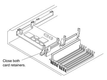
FIGURE 11-8 Closing the SBus Card Retainers
