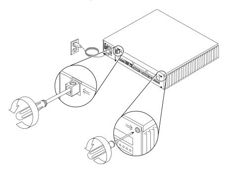
FIGURE 7-1 Removing the Rear Panel Cover Screws
