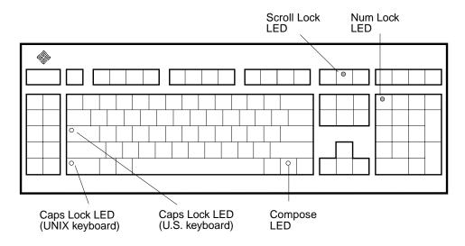
FIGURE 3-1 Arrangement of Sun Type-5 Keyboard Diagnostic LEDs
