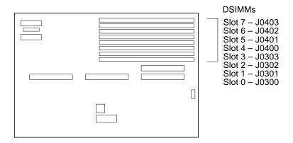
FIGURE 11-14 DSIMM Slot Locations on the System Board
