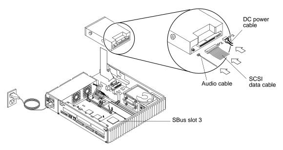
FIGURE 9-6 Replacing the CD-ROM Drive
