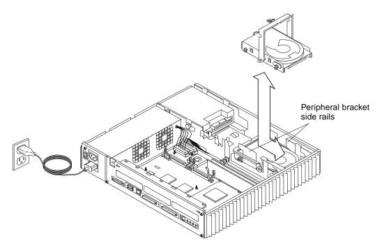
FIGURE 9-3 Replacing a Hard Disk Drive
