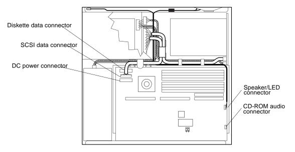
FIGURE 9-18 System Board Cable Connections
