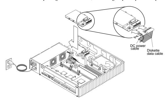
FIGURE 9-11 Replacing the Diskette Drive
