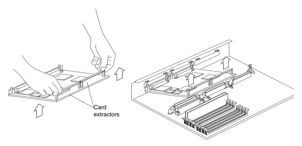
FIGURE 11-6 Removing a Double-Width SBus Card
