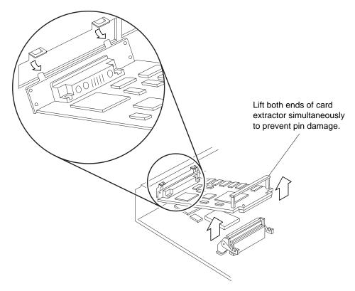
FIGURE 11-11 Removing an S24 Frame Buffer Card
