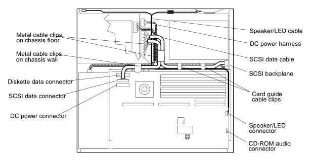
FIGURE 9-21 Internal Cable Routing
