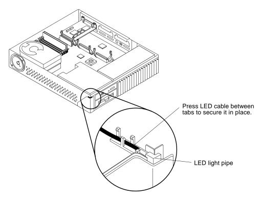
FIGURE 8-4 Routing the LED Cable
