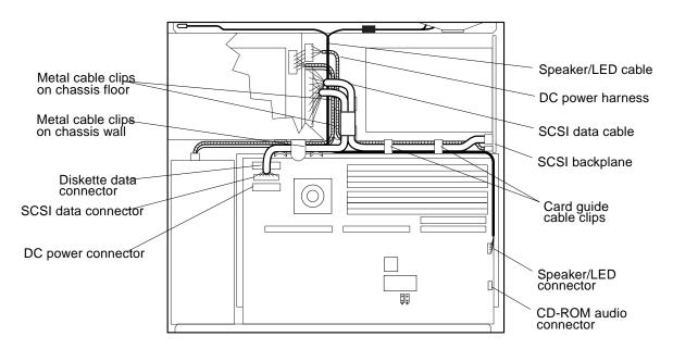
FIGURE 9-15 Internal Cable Routing
