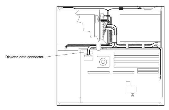
FIGURE 9-24 System Board Cable Routing
