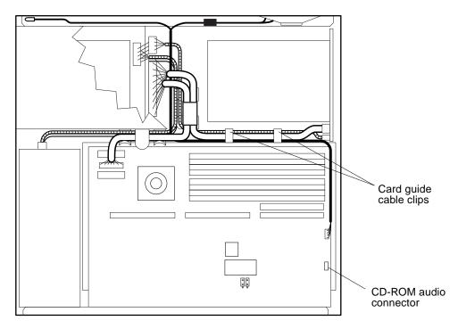
FIGURE 9-26 CD-ROM Audio Connector on the System Board
