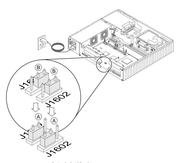
FIGURE 11-23 Setting the Serial Port Jumpers
