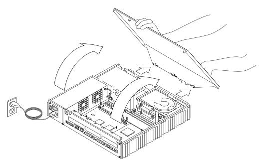
FIGURE 7-2 Removing the Cover
