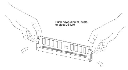
FIGURE 11-15 Ejecting a DSIMM
