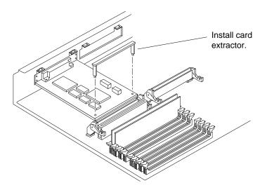
FIGURE 11-4 Installing the SBus Card Extractor
