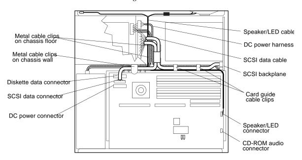
FIGURE 9-12 System Board Cable Connections
