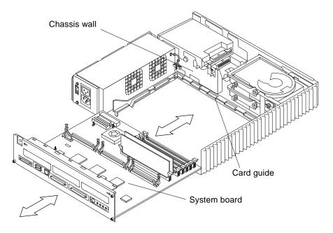
FIGURE 9-22 Replacing the System Board
