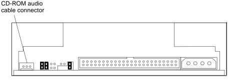
FIGURE 9-25 Audio Cable Connector on the CD-ROM Drive
