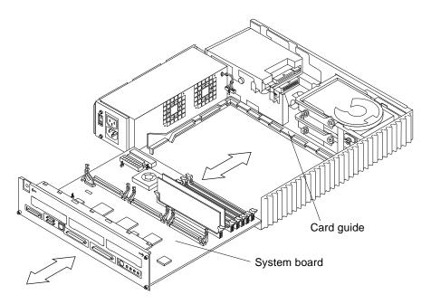
FIGURE 11-21 Installing the System Board
