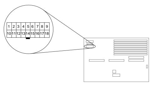
FIGURE 4-1 Power Supply Connector
