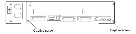
FIGURE 11-22 System Board Captive Screws
