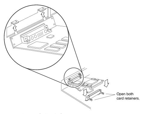
FIGURE 11-7 Inserting the SBus Card
