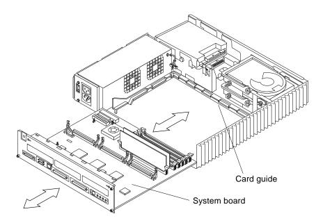
FIGURE 9-14 Removing the System Board
