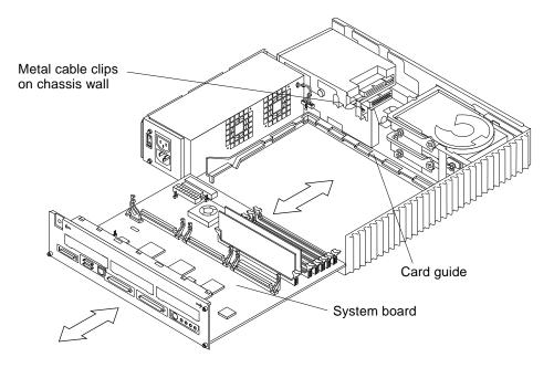
FIGURE 9-16 Replacing the System Board
