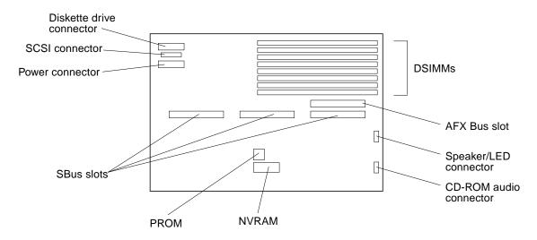
FIGURE 10-1 SPARCstation 5 System Board
