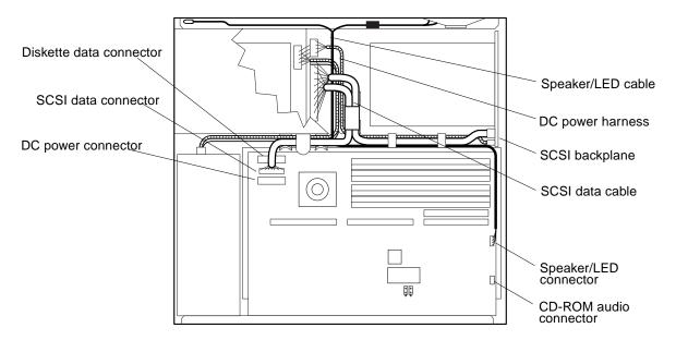
FIGURE 11-18 System Board Cable Connections
