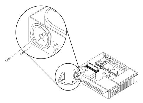
FIGURE 8-6 Removing the Speaker
