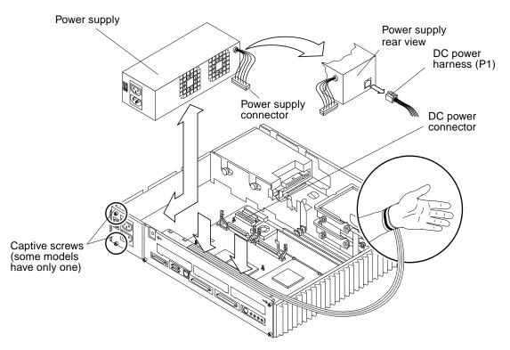
FIGURE 8-1 Removing the Power Supply
