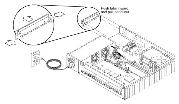
FIGURE 9-8 Removing the CD-ROM Filler Panel
