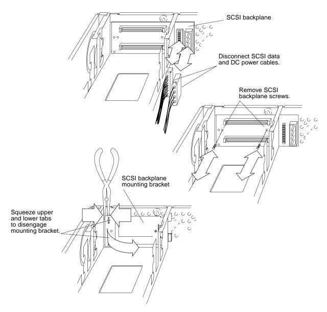
FIGURE 8-8 Removing the SCSI Backplane
