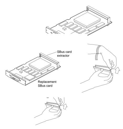
FIGURE 11-3 Removing the Extractor From the SBus Card
