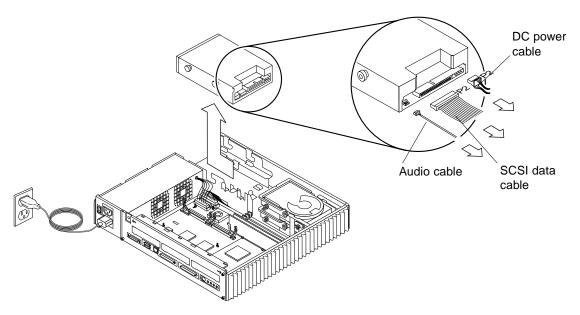
FIGURE 9-4 Removing the CD-ROM Drive
