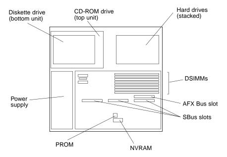
FIGURE 1-2 Interior View of SPARCstation 5 System
