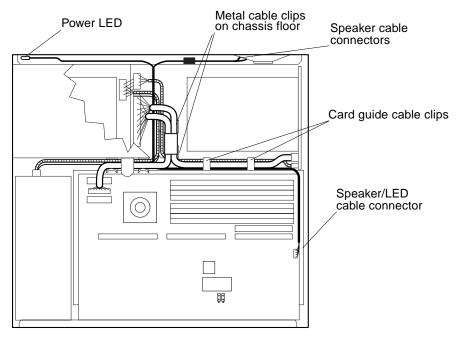
FIGURE 8-3 Speaker/Power LED Cable Connections
