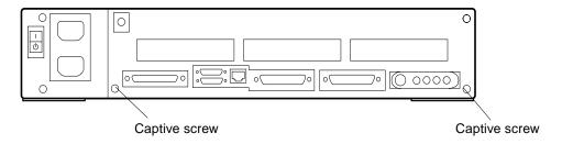
FIGURE 9-19 Rear Panel Captive Screws
