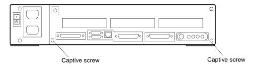
FIGURE 9-23 Rear Panel Captive Screws
