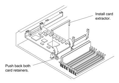
FIGURE 11-10 Opening the Card Retainers
