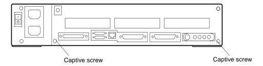
FIGURE 9-13 Rear Panel Captive Screws
