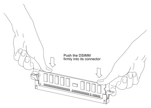
FIGURE 11-17 Installing a DSIMM
