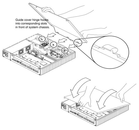
FIGURE 7-4 Replacing the Cover
