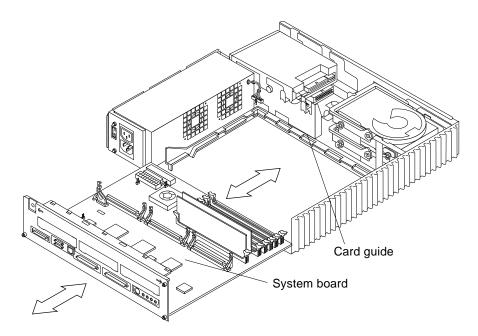
FIGURE 11-20 Removing the System Board
