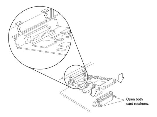
FIGURE 11-12 Inserting an S24 Frame Buffer Card
