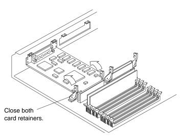
FIGURE 11-13 Closing the Card Retainers
