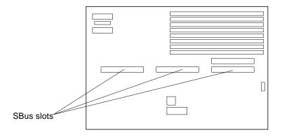
FIGURE 11-1 SBus Slot Locations
