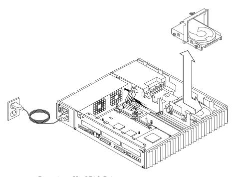
FIGURE 9-2 Removing a Hard Disk Drive
