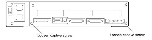
FIGURE 11-19 System Board Captive Screws
