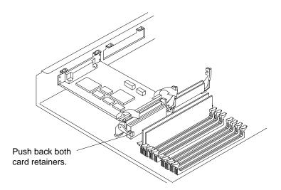
FIGURE 11-2 Opening the SBus Card Retainers
