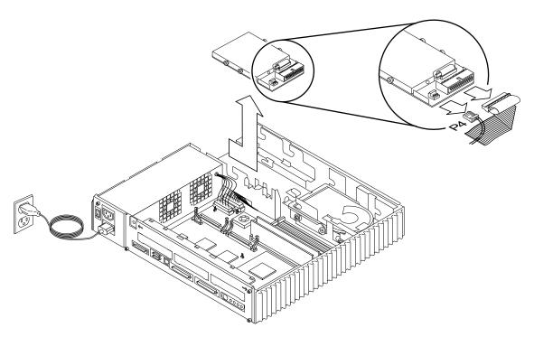
FIGURE 9-10 Removing the Diskette Drive
