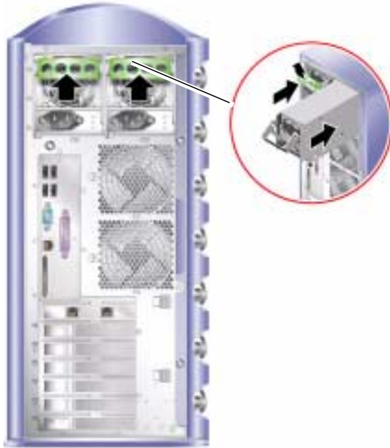
FIGURE 1-9 Replacing A Power Supply Unit
