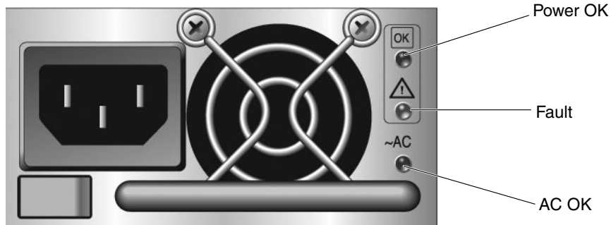
FIGURE 3-5 Power Supply LEDs
