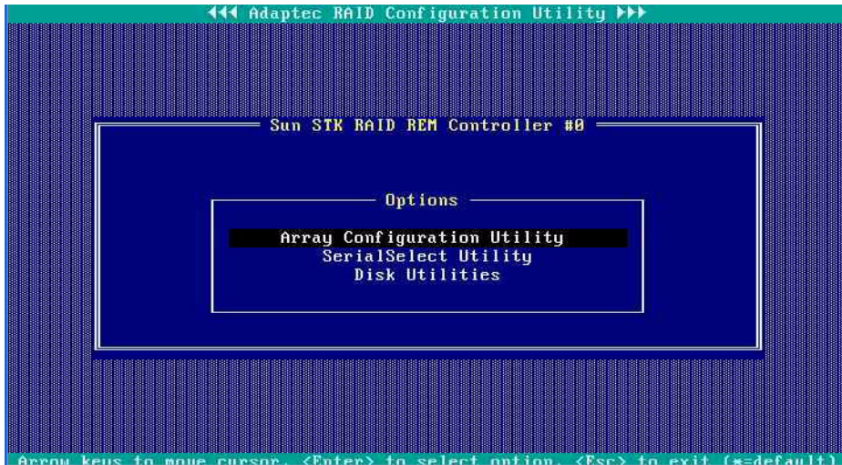
FIGURE 8-1 Opening Screen of the Adaptec RAID Configuration Utility (ARCU)
