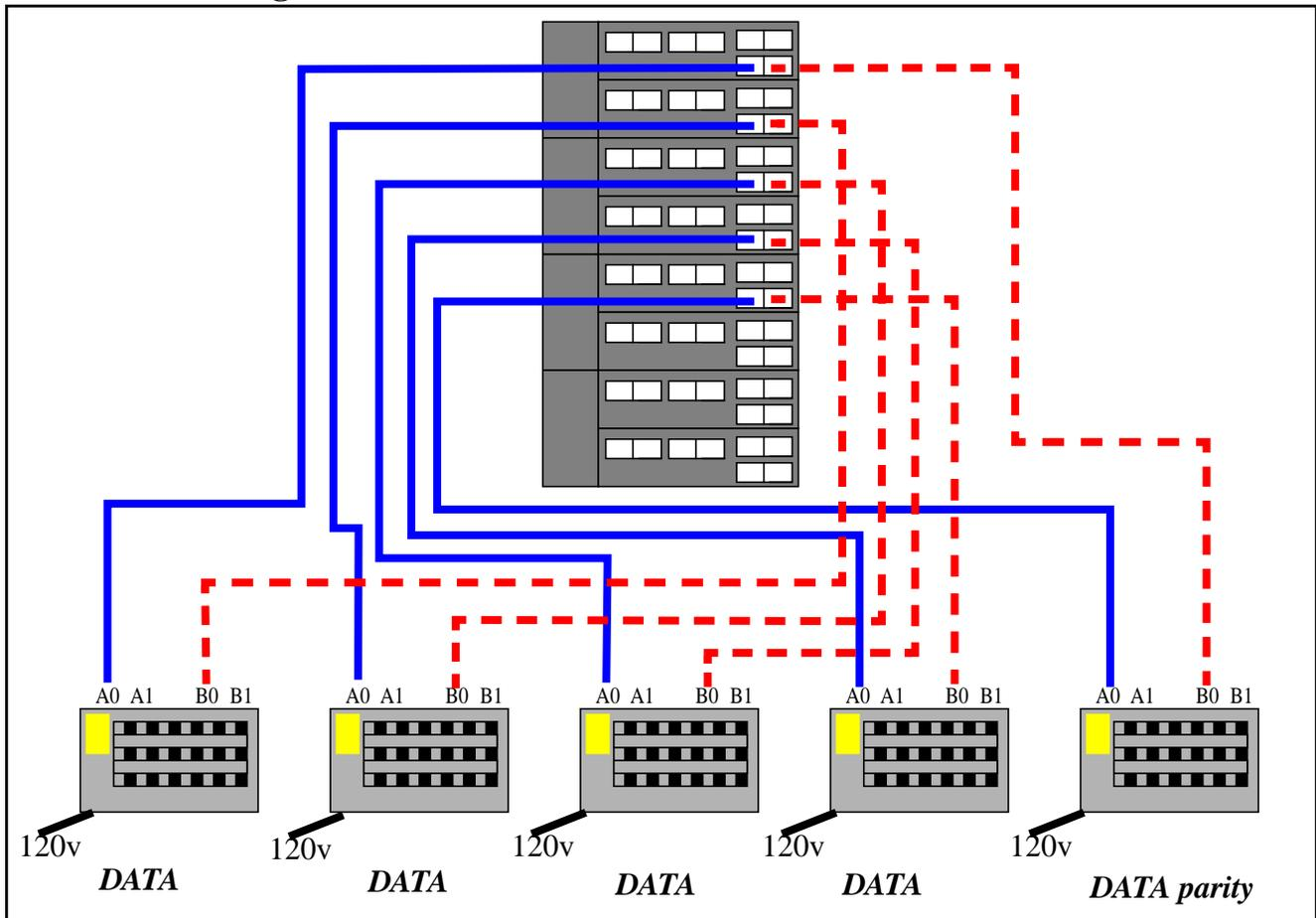
Note: The example above depicts RAID5 with 4 data disks and one parity disk (4+1). RAID5 actually stripes parity across all disks, but the example is used for simplicity. Also note that the server requires 5 system boards, one for each array. For very large installations the above configuration could be built using racks instead of table top arrays.
