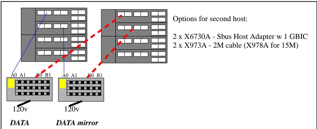
Note: The second host would connect to the B0 array ports. This gives better fault tolerance and performance as data traffic or errors on one host's loop will not effect the other host.
