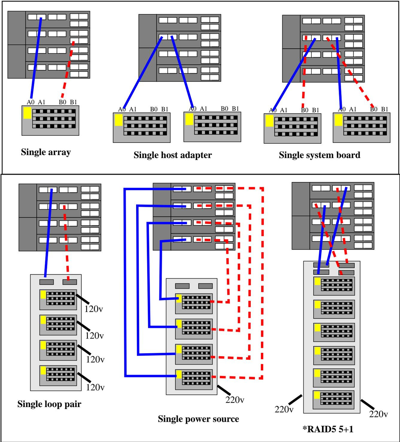
\* For this RAID5 example, although this would be an excellent mirror config, you would need two more racks (6 redundant array groups) to implement a fully redundant RAID5 5+1 configuration.
