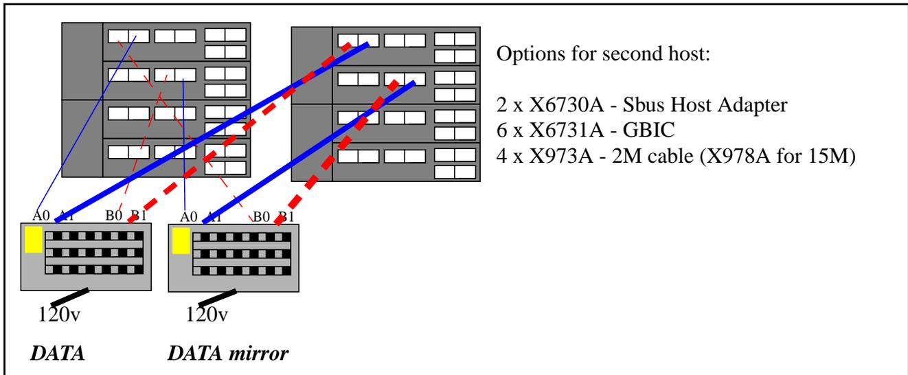
Note: For hosts that use an array disk for booting you should configure one host to boot to loop A, the other host to boot to loop B. This will prevent data traffic or errors from one host effecting the other.
