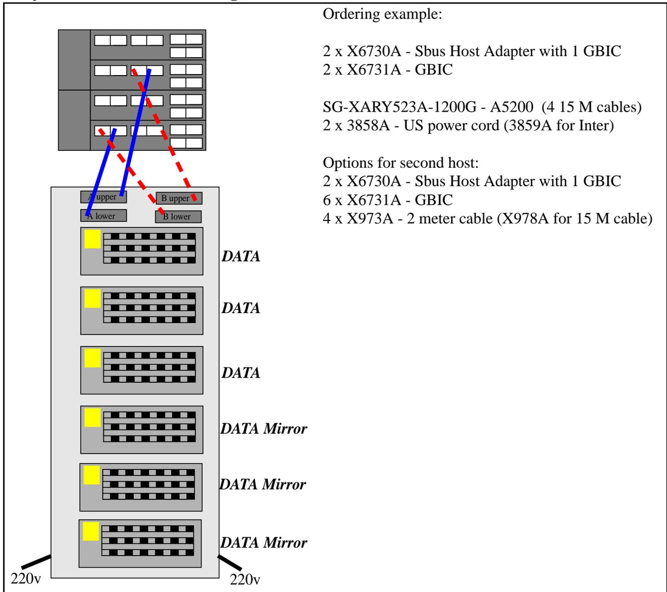
This fully redundant mirrored rack configuration is much simpler to implement. The disadvantage over the Best direct connect rack example is that one failure can take out 3 array mirrors (such as a dual loop error caused by a failed mother board). After the failure is resolved the mirrors will require a fully resync which will take many hours. A similar failure for direct connect would only effect 2 arrays not 6.
