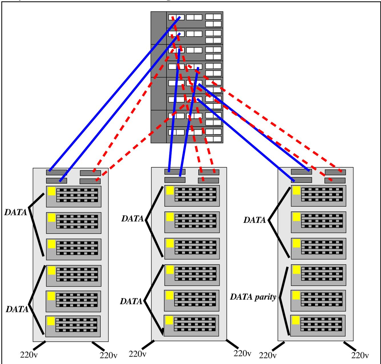
This example shows use of both the A and B loops, this is not a requirement for full redundancy, but is highly recommended as the slight extra cost yields greater fault tolerance and performance.
