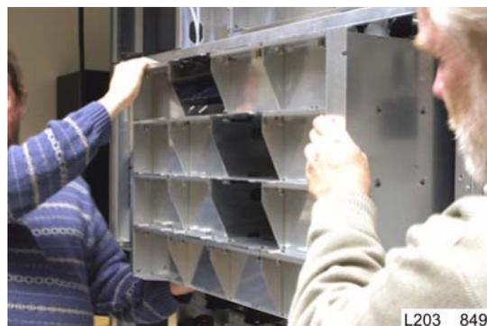
12. Slide the drive array out of the library and place it on a work surface.
