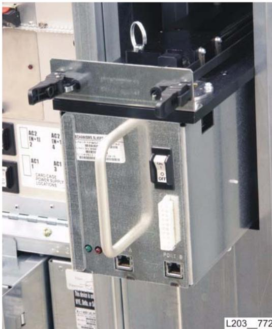
7. Slide the PTP mechanism from the library and place it out of the work area.
