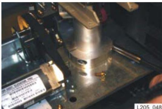
6. Remove the two T15 screws that hold the upper tube clamp in place.
