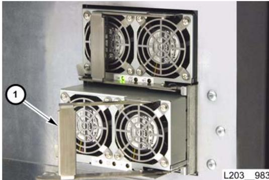
1. Push the replacement power supply, with the handle (1) extended, fully into the slot until the connectors are seated.
