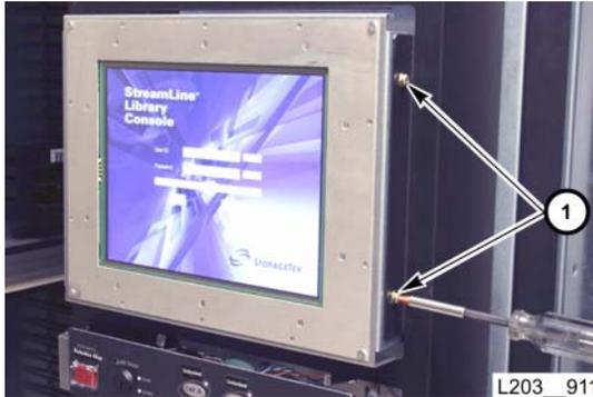
1. Support the panel in the mount and align with the mounting slots.
