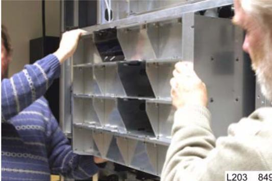
**WARNING:** *Lifting hazard:* The upper drive array weights approximately 34kg (75 lb). Follow the directions in “**Lifting Techniques.**”
