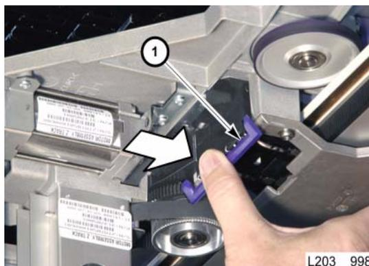
11. Remove the rail brush locking lever shipping tape, if present.
