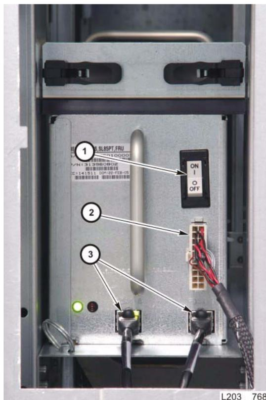
2. Set the PTP mechanism power switch (1) to OFF.
