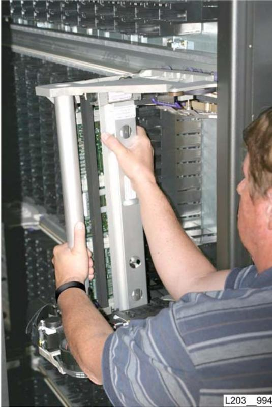
**CAUTION:** *Possible Equipment Damage:* Do not grasp or bump the lower plate or any plastic parts on the HandBot during removal. Lift the HandBot Z-column and frame only.
