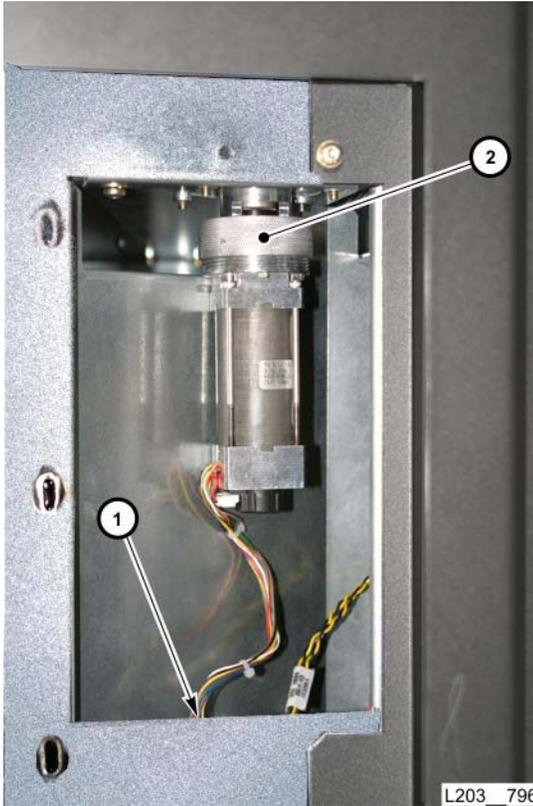
1. Position the replacement motor assembly into the mounting area, making sure the motor shaft coupler tab is aligned with the linkage coupler slot.
