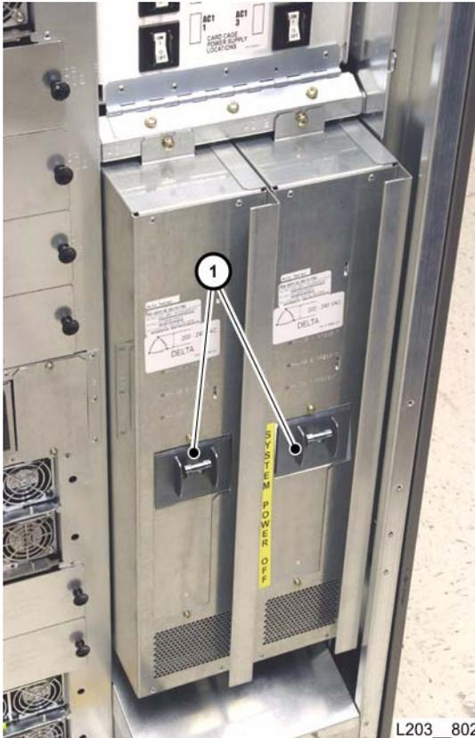
7. Set PDU circuit breaker(s) (1) to ON (up).
