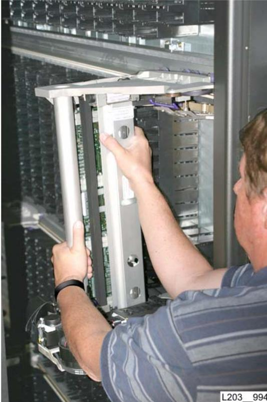
**WARNING:** *Electrical Shock Hazard:* There is 48 VDC present on the electrical bar of powered rail assemblies (in the case of a service safety door activation). **DO NOT TOUCH** the electrical bar during the remaining steps.
