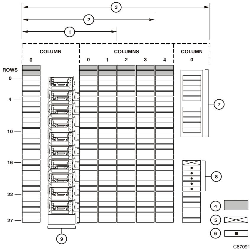
**Figure 3-1. L180 Cartridge-Cell Arrays, CAP, and Drive Column (Continued)**
