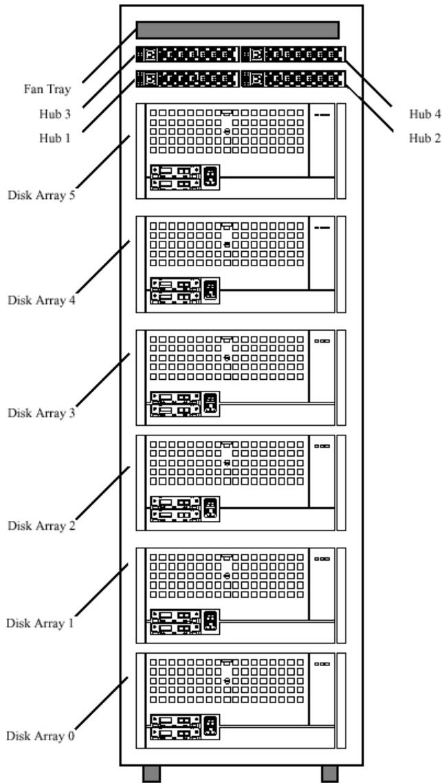
**Figure 11.** Rackmounting the Sun StorEdge A5X00 system
