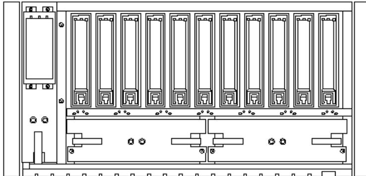
Figure 6. Front components
