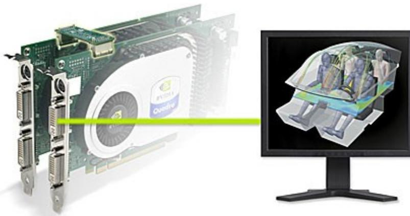
**2. SLI Multi View:** Combines the power of two NVIDIA Quadro PCI Express graphics cards to span a single hardware-accelerated OpenGL application window across multiple displays, run a single application per GPU with multiple display outputs, or enable other flexible usage of two PCI Express graphics cards.
