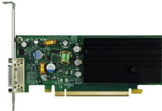
The NVIDIA Quadro NVS 285 128 MB DDR-2 (PCI Express) Graphics card is a professional 2D graphics card with dual-display capabilities. The Sun Ultra 40 M2 Workstation supports up to four NVIDIA Quadro NVS 285 DDR2 graphics cards and can drive up to eight displays, two per board. This card ships with 128MB of DDR memory and can drive up to two Sun 17-inch LCD monitors, two Sun 20.1-inch LCDs, two Sun 19-inch TFT LCD monitors, or two Sun 24.1-inch LCD.
