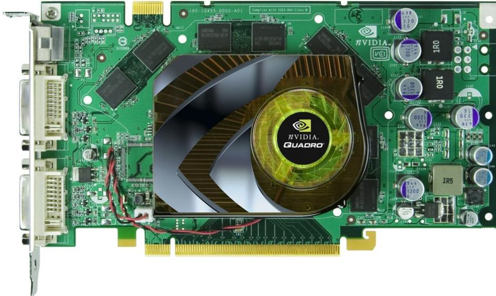
The NVIDIA® Quadro® FX 1500 graphics card provides Sun customers a mid-range 3D performance workstation graphics solution for professional MCAD applications. The Sun Ultra 40 M2 Workstation supports up to four NVIDIA Quadro FX 1500 graphics cards. This card ships with 256MB of DDR memory and can drive any two Sun displays, including two 24.1-inch LCD monitors.
