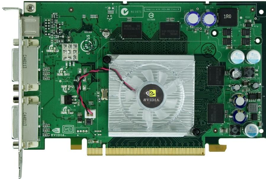
The NVIDIA® Quadro FX 560 graphics card provides Sun customers an entry-level 3D performance workstation graphics solution for SW development or everyday MCAD applications. This card ships with 128MB of DDR memory and can drive two Sun LCD displays .
