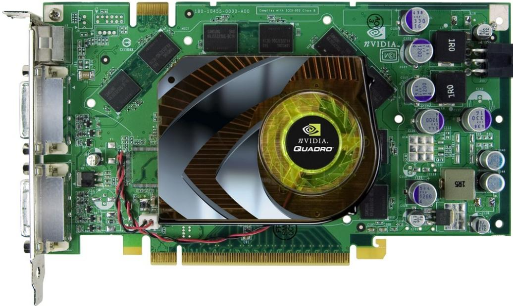
The NVIDIA Quadro FX 3500 graphics card provides Sun customers a high-end 3D performance workstation graphics solution for professional MCAD. The Sun Ultra 40 M2 Workstation supports up to four NVIDIA Quadro FX 3500 graphics cards with NVIDIA SLI technology. This card ships with 256MB of DDR memory and can drive any two Sun displays, including two 24.1-inch LCD monitors.
