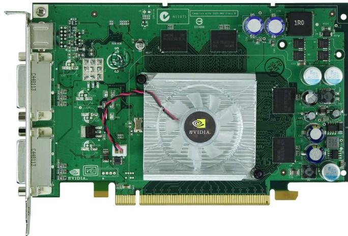
Figure 14 – Board Layout of the NVIDIA Quadro FX 560 Graphics Accelerator Card
