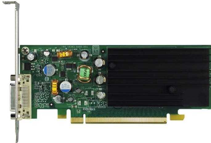
Figure 17 –Board Layout of NVIDIA Quadro NVS 285 Graphics Accelerator Card
