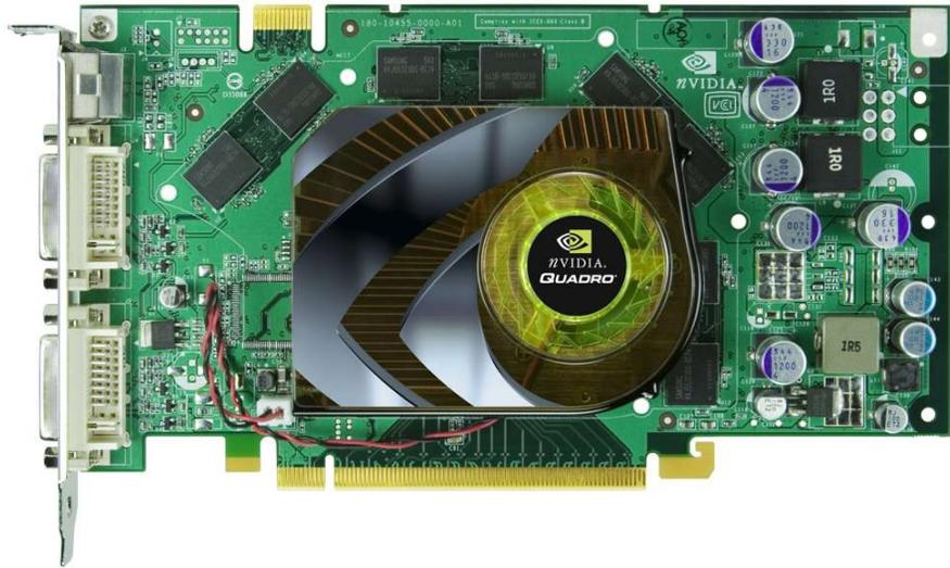
Figure 12 – Board Layout of NVIDIA Quadro FX 1500 Graphics Accelerator Card
