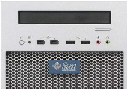
Figure 6 – Front I/O Ports of Sun Ultra 20 M2 Workstation
