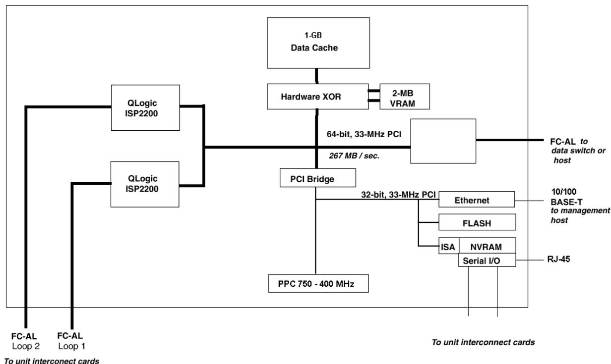
**Figure 4.** Controller architecture
