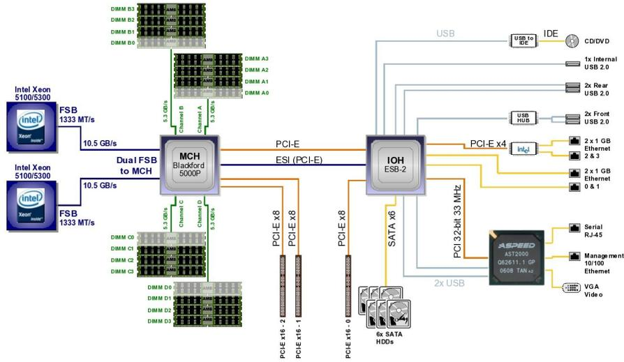
Figure 3. Sun Fire X4450 SATA Server Block Diagram
