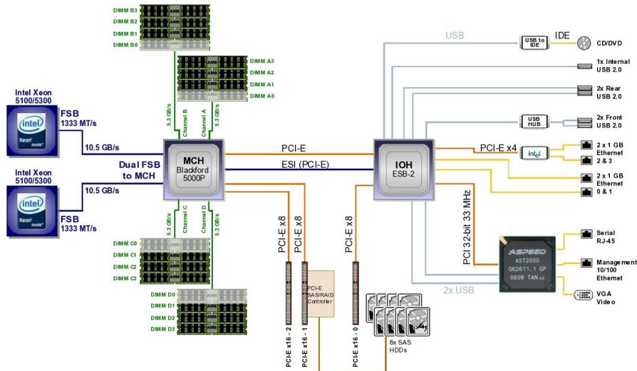
Figure 4. Sun Fire X4450 SAS Server Block Diagram
