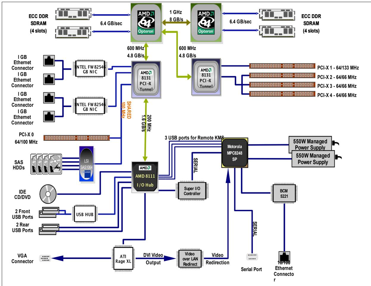
Figure 11.Sun Fire X4200 Server Block Diagram
