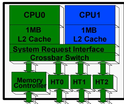
Figure 1. Opteron Dual-Core Processor Architecture
