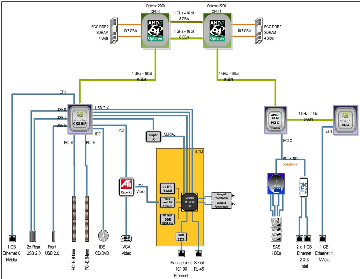
Figure 12. Sun Fire X4100 M2 Server Block Diagram
