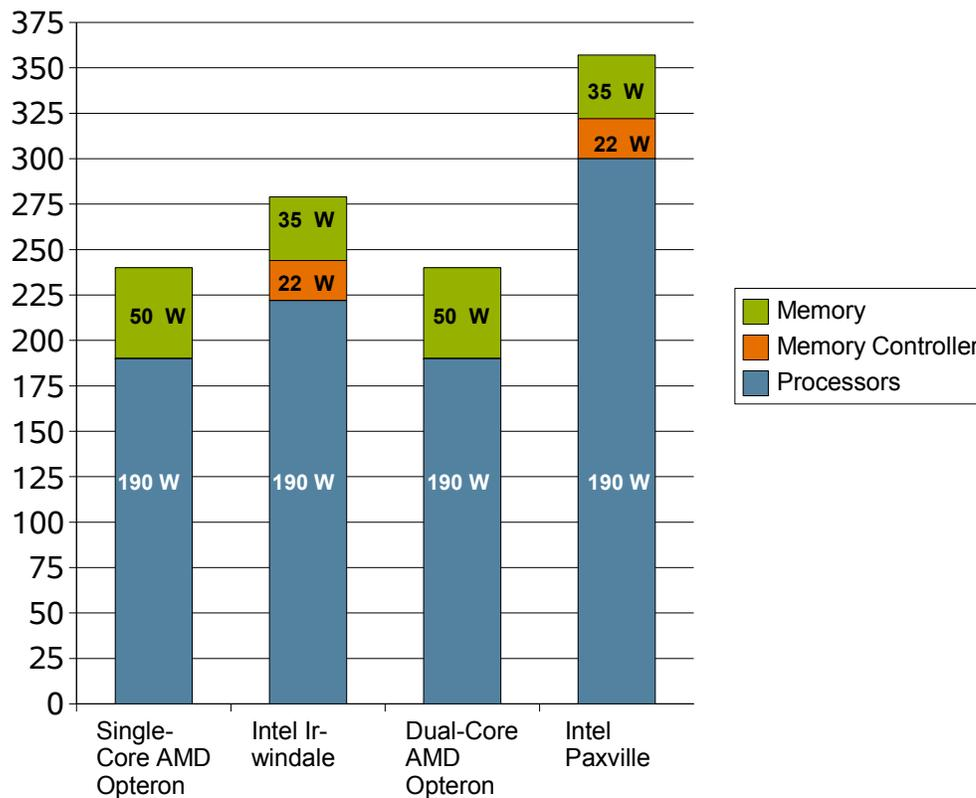
Figure 7. Current Product Processor, Memory Controller & Memory Power Requirements
