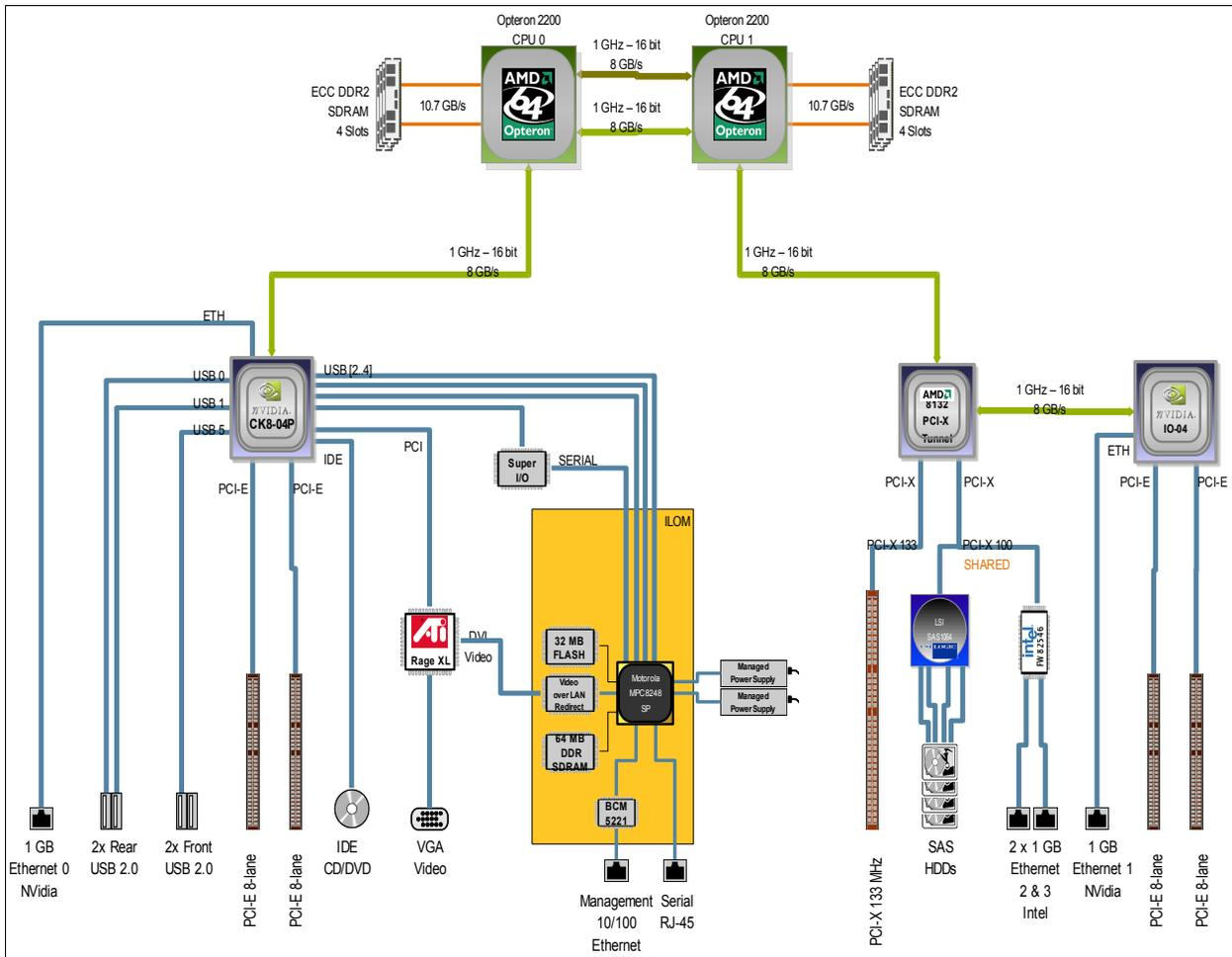
Figure 13. Sun Fire X4200 M2 Server Block Diagram
