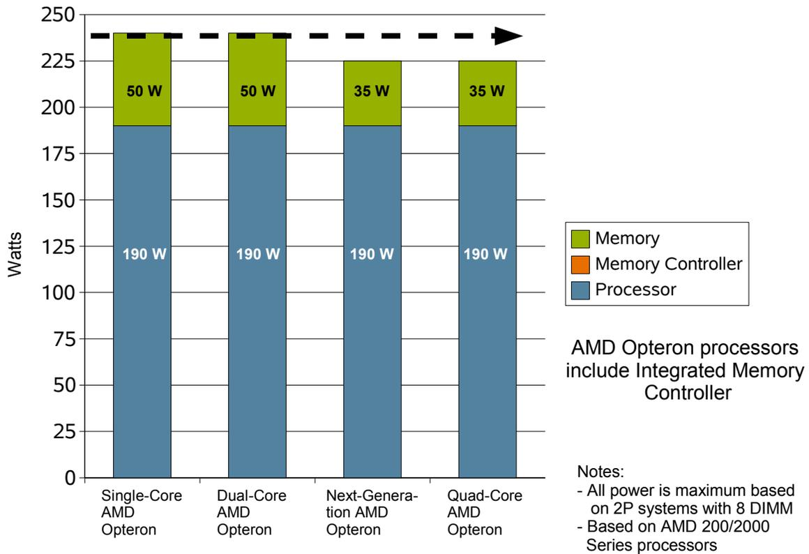
Figure 5. Processor, Memory Controller and Memory Power Requirements
