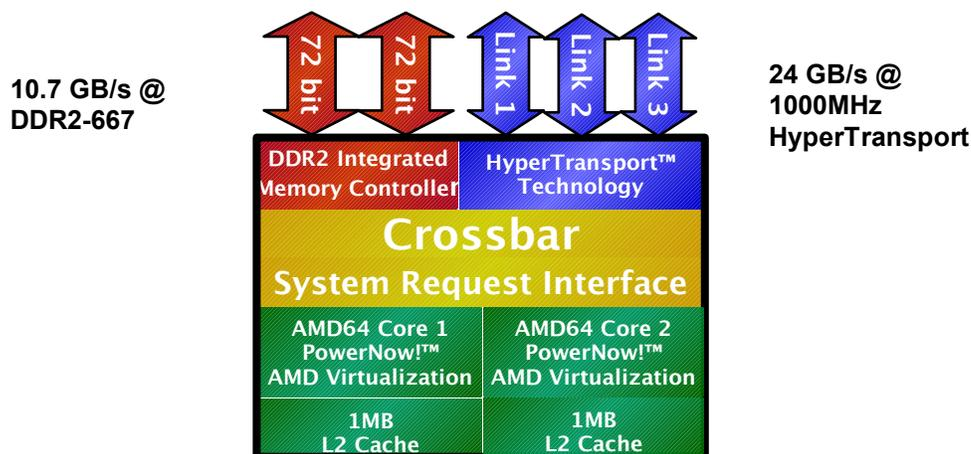
Figure 2. Next-Generation AMD Opteron Processor Design for Socket F (1207)
