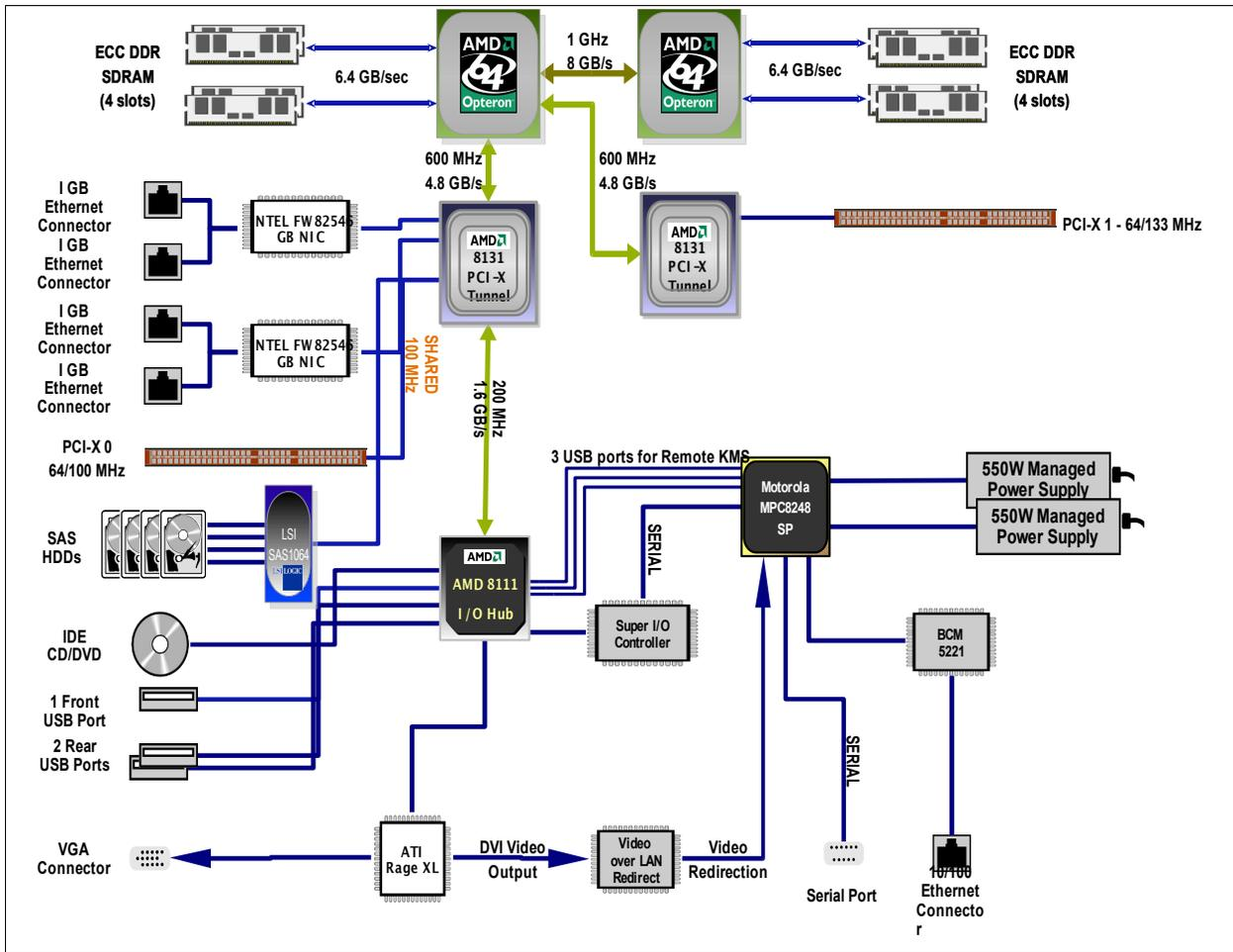
Figure 10. Sun Fire X4100 Server Block Diagram
