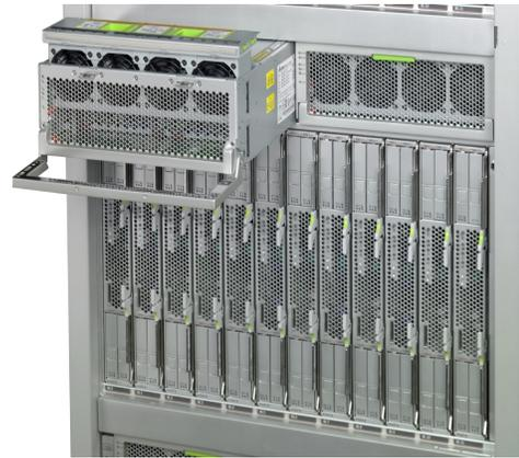
**Integrated Fan Module Removed**
