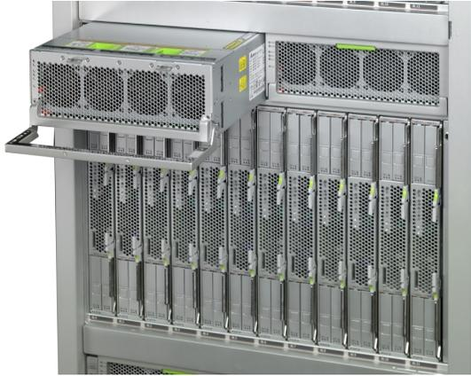
**Power Supply Module Removed**
