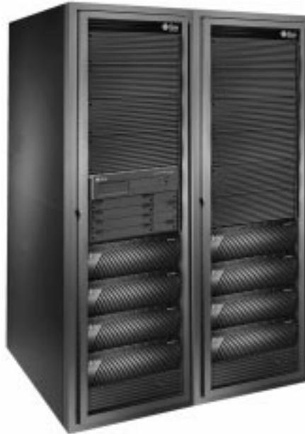
**Figure 1.** Sun StorEdge™ N8600 filer in two-cabinet configuration
