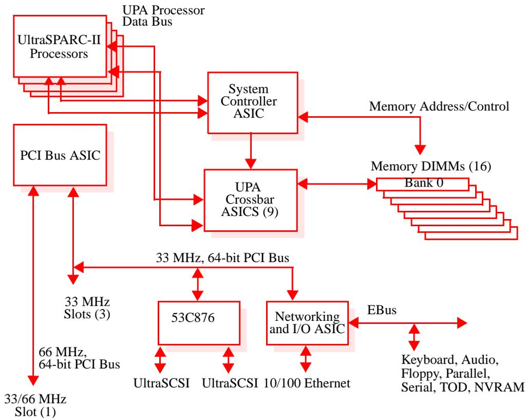
**Figure 2.** Architecture of the Sun Enterprise 420R server system
