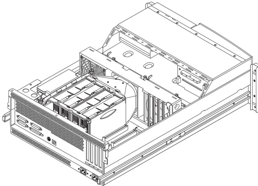
**Figure 3.** Sun Enterprise 420R server chassis with access panel removed, provides full access to internal options
