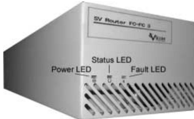
**Figure 4-1** Front Panel SV Router FC-FC 3 - LED Locations
