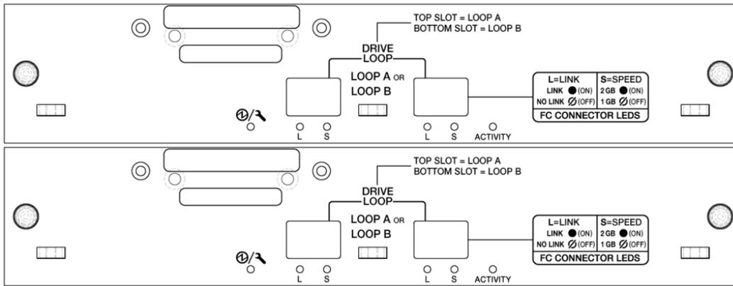
**Figure 8.** Expansion-I/O modules, Sun StorEdge 3510 Fibre Channel array
