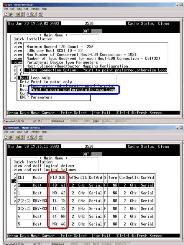
Figure 9. Configuration menu for private loop or point to point mode
