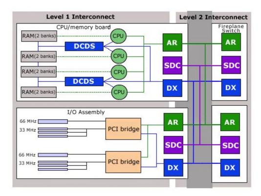
Figure 7 - Logical view of Sun Fire 3800-6800 system
