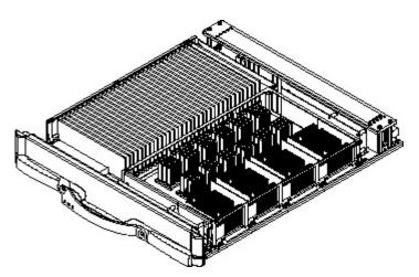
Figure 10 - Sun Fire 3800-6800 CPU/memory board (processor/e-cache cover has been removed)
