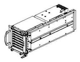
Figure 12 - 8-slot PCI I/O assembly
