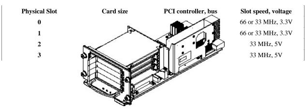
Figure 16 - 4-slot CompactPCI I/O assembly
