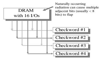
Each Checkword is 128 + 16 bits long and is capable of correcting a single bit or detecting double bit error
