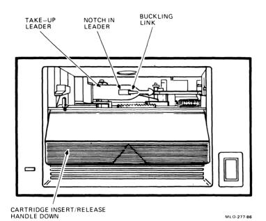
If the leader is unhooked or if you cannot clearly see the pointed end, DO NOT INSERT THE CARTRIDGE INTO THE DRIVE. DO NOT ATTEMPT TO FIX THE LEADER. Contact your service representative.
