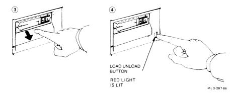
5. The tape loads in 10-15 seconds. During loading the two leaders couple and the tape winds onto the take-up reel inside the tape drive.
