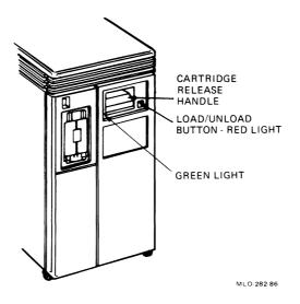
To operate the drive properly, you must carefully monitor the status lights. The instructions for inserting/removing cartridges later in this section tell you exactly what should happen at each step. A table at the end of the section summarizes light and control combinations.
